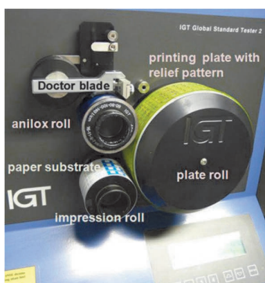
Figure 6. The flexographic printing unit.
