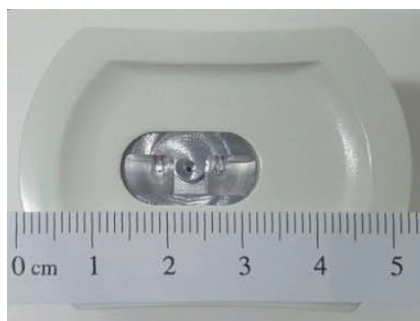
Figure 11. The handheld NIR probe (Spectral Engines Oy, Helsinki, Finland).
