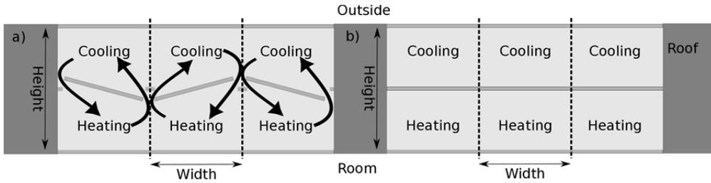
Figure 2. Developed skylight design in cooling mode a) and in insulating mode b) (Paper V)
