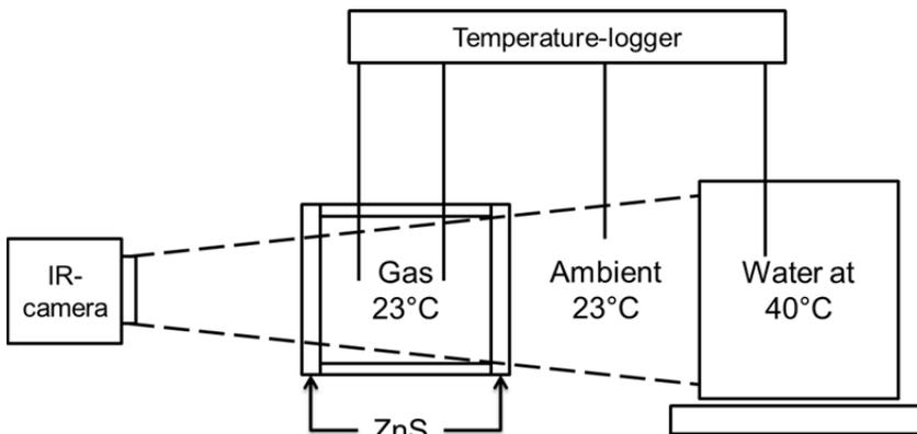
Figure 20. Experimental setup for material suitability testing (Paper VI)
