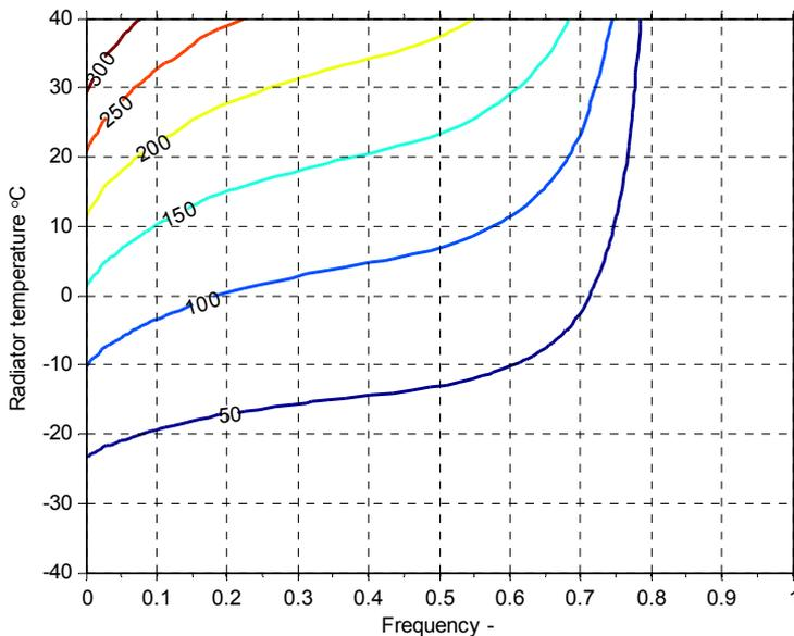
Figure 12. Cumulative frequency distribution of radiative heat exchange in W/m<sup>2</sup> at different radiator temperatures in Helsinki (Paper II)
