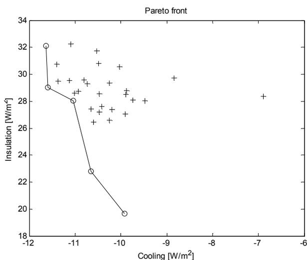
Figure 16. Results from optimization: a) The Pareto front is noted with “o” and the inferior solutions are marked with “+” (Paper V)
