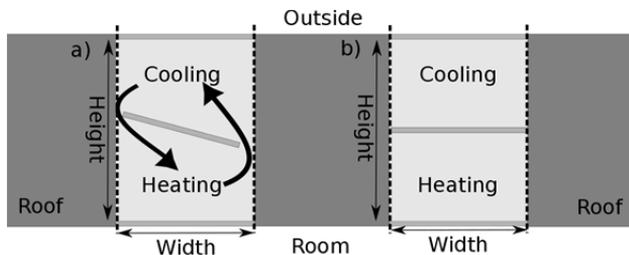
Figure 1. Initial skylight design in cooling mode a) and in insulating mode b) (Paper V)
