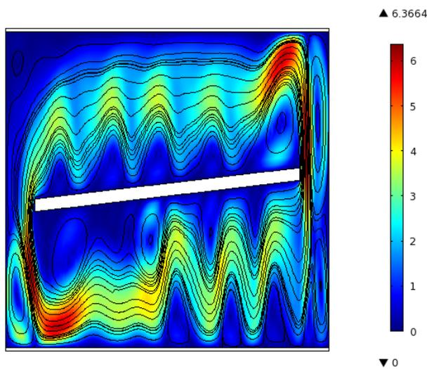
Figure 13. Velocity profile in (cm/s) for cooling mode during summer (Paper III)
