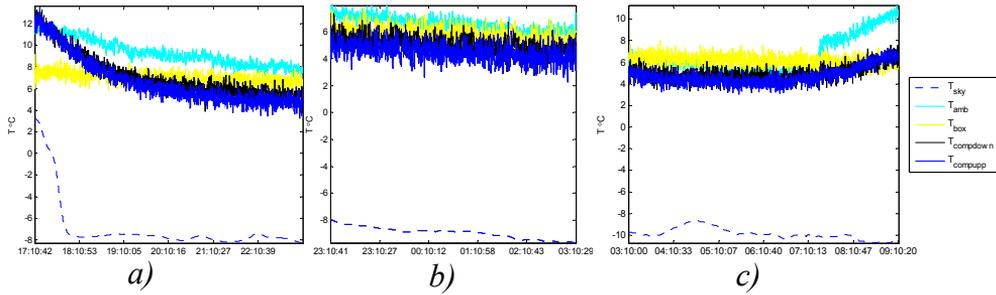
Figure 24. Temperature profiles from the experiment with: a) CO<sub>2</sub>; b) Air, c) HFC-125 (Paper VI)
