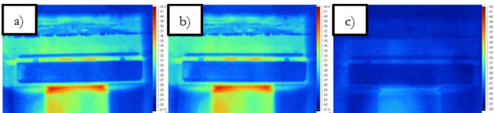
Figure 21. Thermal images of the skylight filled with a) air; b) CO<sub>2</sub>; c) HFC-125 (Paper VI)
