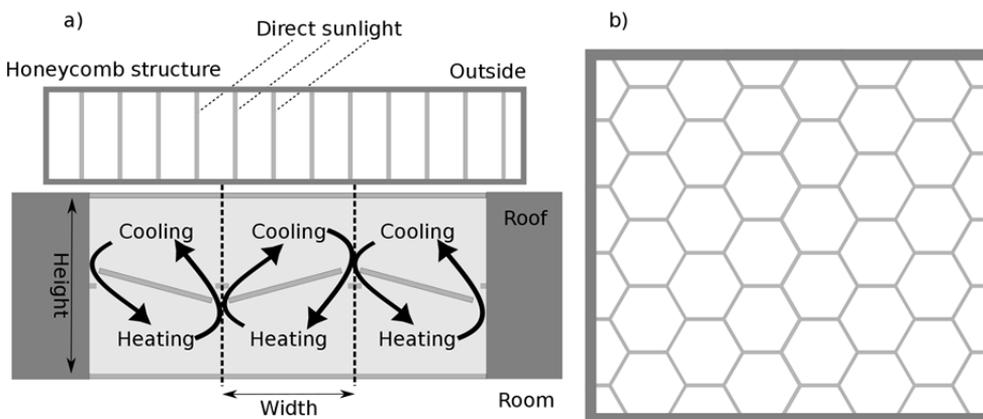
Figure 25. A schematic presentation of the intended honeycomb structure, a) side view of the skylight and the honeycomb structure, b) view from beneath the skylight
