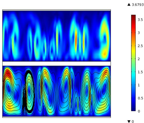
Figure 14. Velocity profile in (cm/s) for insulating mode during winter (Paper III)
