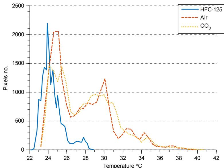
Figure 22. The number of pixels in the pictures in Fig. 6 taken with the thermal imager at a particular temperature (Paper VI)
