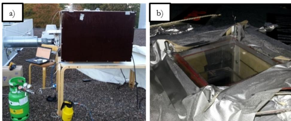
Figure 23. Experimental set-up for the second and third set of experiments: a) the total set-up, showing the dark sidewall of the “room”; b) the top of the skylight (Paper VI)
