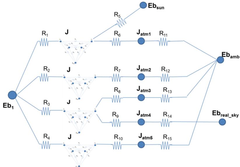
Figure 18. Resistance network for wavelength radiation model (Paper IV)
