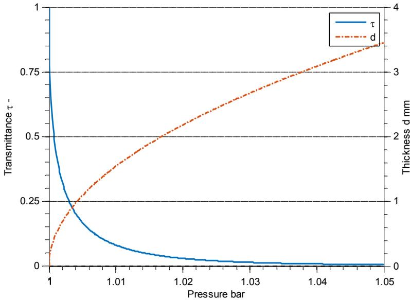
Figure 8. Transmittance  $\tau$  and thickness  $d$  of an HDPE window at increasing pressures (Paper I)
