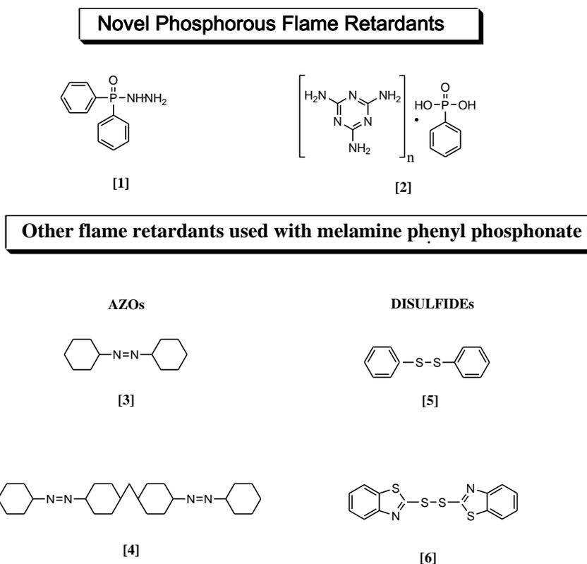
**Figure 7:** Molecular structures of P'P-diphenyl phosphinic hydrazide (1), melamine phenyl phosphonate (2), azocyclohexane (3), 4'4-bis(cyclohexylazocyclohexyl) methane (4) diphenyl disulfide (5) and 2'2'-dithiobis-benzothiazole (6).
