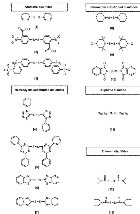
Figure 5: Chemical structures of investigated disulfides.
