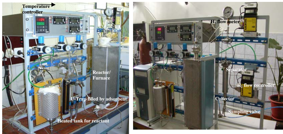
Figure 3.4. Reactor set-up for fixed bed hydrogenation (Boreskov Institute of Catalysis).
