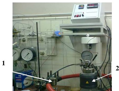
Figure 3.3. Laboratory set-up for oil hydrogenation (BIC, Russia).
