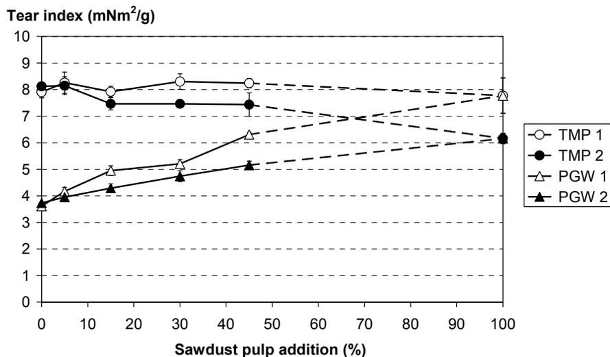
Figure 25. Tear index of the different pulp furnishes.
