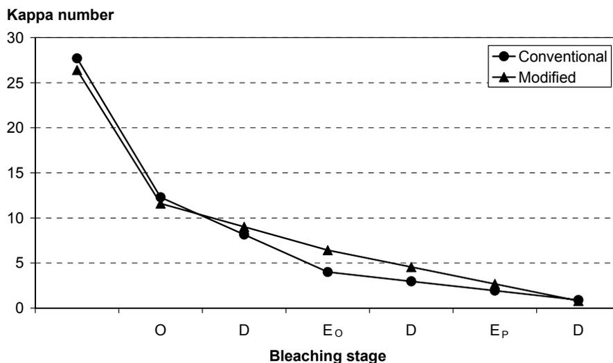
Figure 15. Kappa number as a function of the bleaching stage.
