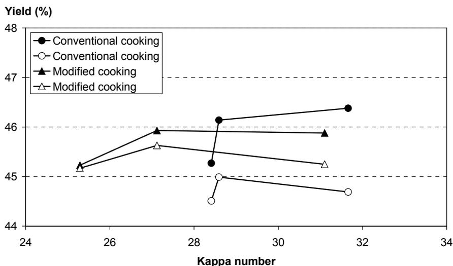
Figure 14. Total (solid symbol) and screened yield (hollow symbol) as a function of kappa number.
