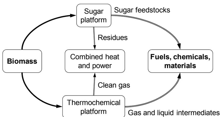
Figure 5. Biorefinery concept, redrawn from Crocker and Crofcheck 2006.
