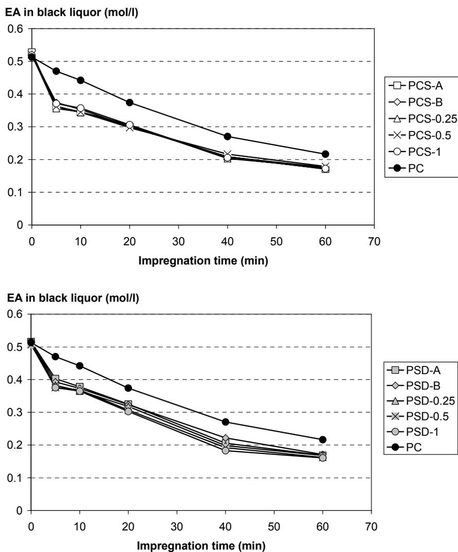
Figure 10. Effective alkali (EA) of the black liquor drained from the impregnation of pine chip screenings (PCS, upper), pine sawdust (PSD, lower) and pine chips (PC, upper and lower) as a function of time.
