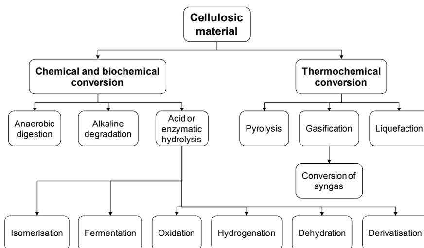
Figure 6. Conversion of cellulosic materials, redrawn from Alén 1990.
