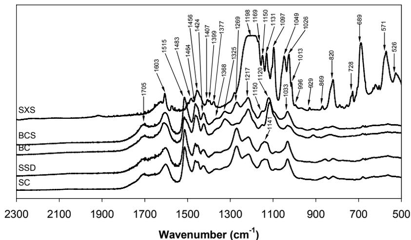
Figure 22. FT-IR absorbance spectra of precipitated lignin samples and SXS. Spectra of SXS: sodium xylenesulphonate, BCS: Nordic birch chip screenings, BC: Nordic birch chips, SSD: Norway spruce sawdust, SC: Norway spruce chips.
