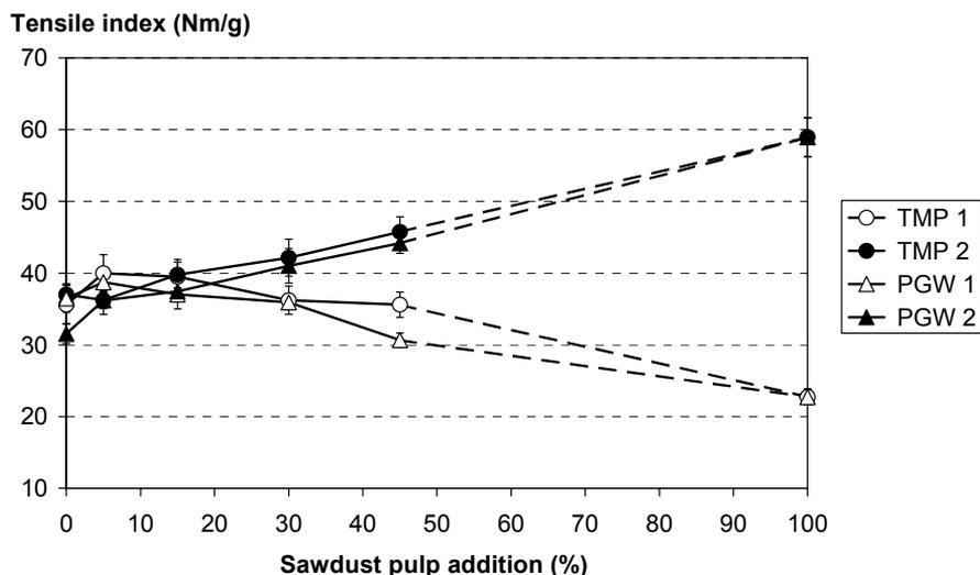
Figure 26. Tensile index of the different pulp furnishes.
