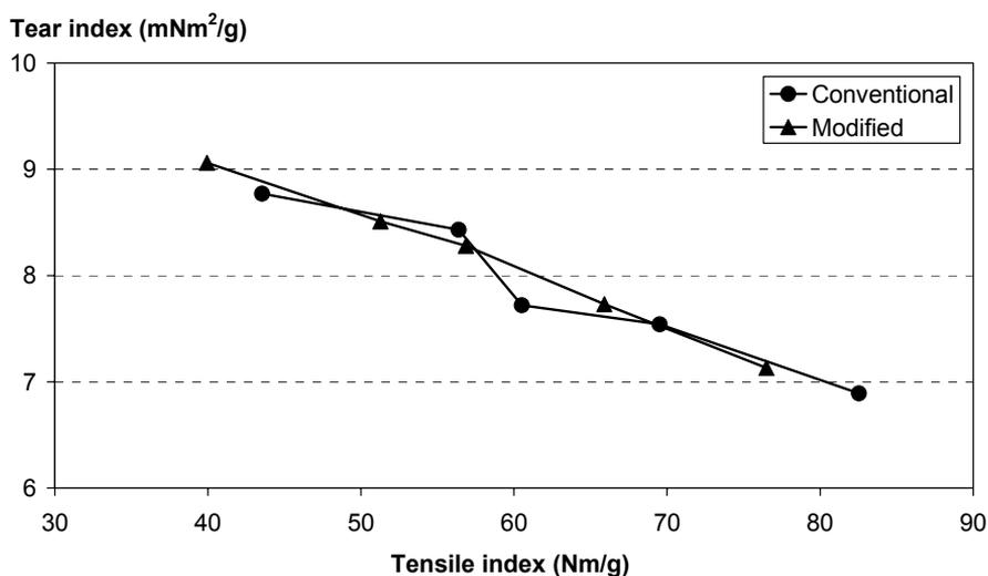
Figure 18. Tear index as a function of tensile index.
