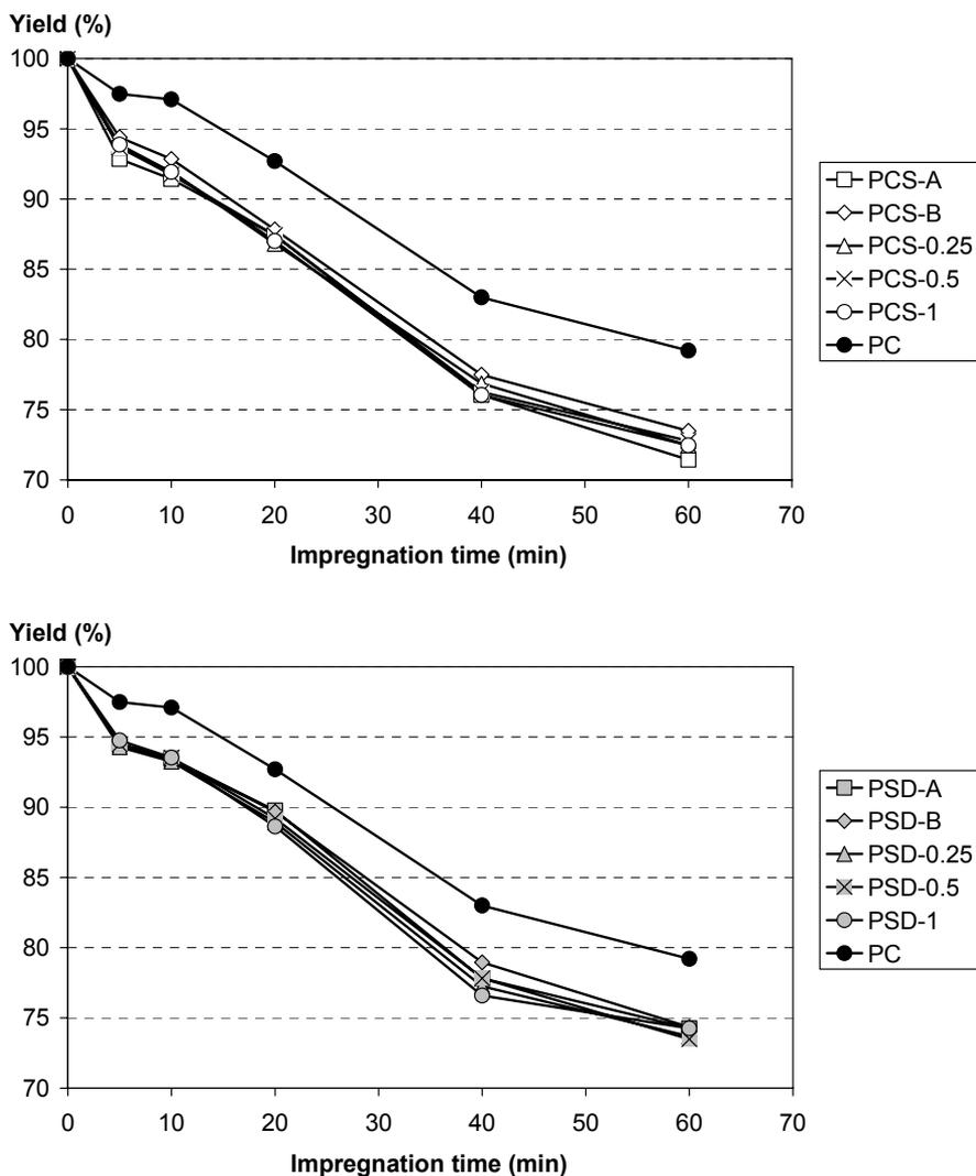
Figure 12. Wood yield after impregnation of pine chip screenings (PCS, upper), pine sawdust (PSD, lower) and pine chips (PC, upper and lower) as a function of time.
