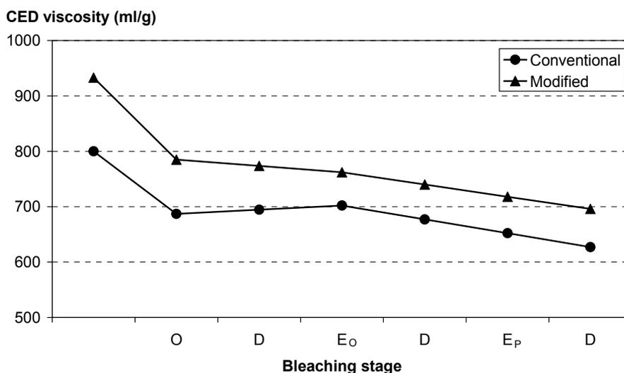
Figure 16. Intrinsic viscosity as a function of the bleaching stage.
