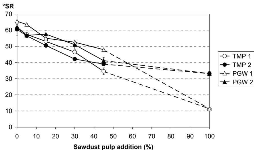
Figure 23. Drainability of the different pulp furnishes. TMP 1: Bleached thermomechanical pulp blended with bleached, unrefined sawdust kraft pulp, TMP 2: Bleached thermomechanical pulp blended with bleached, refined sawdust kraft pulp, PGW 1: Bleached pressurised groundwood pulp blended with bleached, unrefined sawdust kraft pulp, PGW 2: Bleached pressurised groundwood pulp blended with bleached, refined sawdust kraft.
