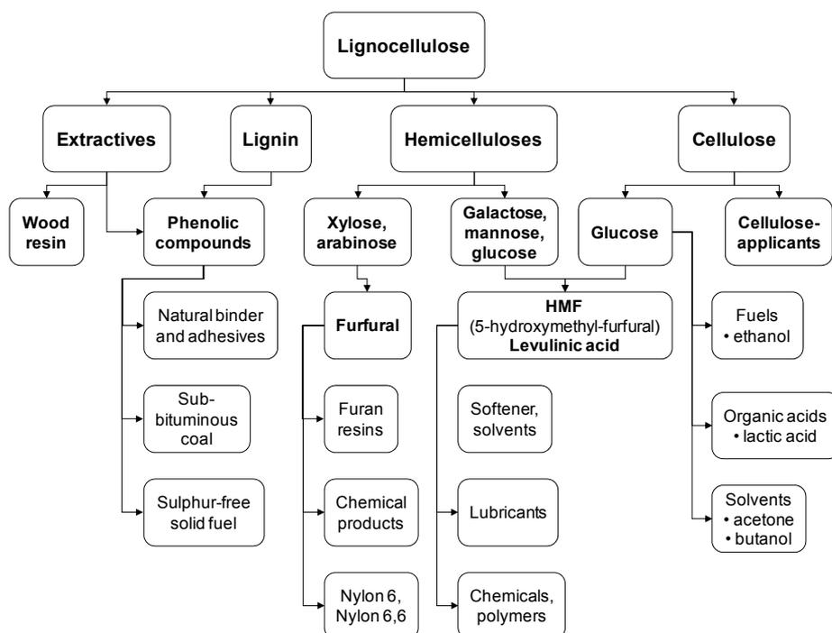
Figure 9. Composition of lignocellulosic materials and converted products, redrawn from Kamm and Kamm 2004; Taherzadeh and Keikhosro 2007.
