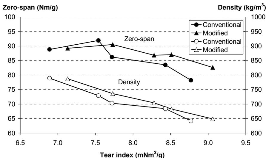
Figure 19. Zero-span tensile strength (solid symbol) and apparent sheet density (hollow symbol) as a function of the tear index.
