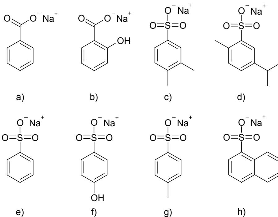
Figure 4. Hydrotropic sodium salts: a) sodium benzoate, b) sodium salicylate, c) sodium xylenesulphonate, d) sodium cymenesulphonate, e) sodium benzenesulphonate, f) sodium phenolsulphonate, g) sodium toluenesulphonate and h) sodium naphthalenesulphonate. Only one isomer of the all possible isomers is shown.
