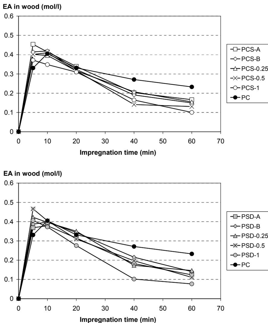
Figure 11. Effective alkali (EA) released from wood during impregnation in pine chip screenings (PCS, upper), pine sawdust (PSD, lower) and pine chips (PC, upper and lower) as a function of time.
