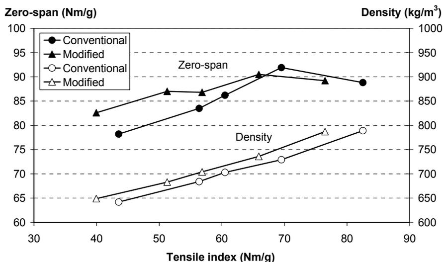
Figure 20. Zero-span tensile strength (solid symbol) and apparent sheet density (hollow symbol) as a function of the tensile index.
