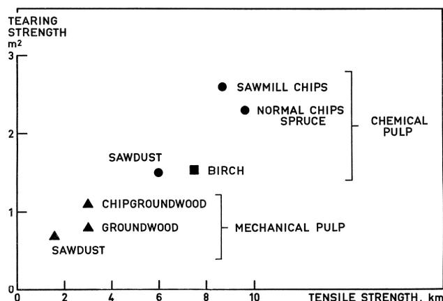
Figure 7. Strength properties of different pulps (Lönnberg 1971).
