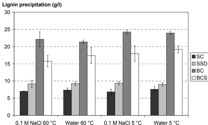
Figure 21. Lignin precipitation from spent hydrotropic extraction solution. SC: spruce chips, SSD: spruce chip screenings, BC: birch chips, BCS: birch chip screenings.
