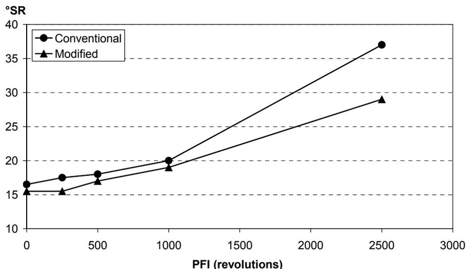
Figure 17. Schopper-Riegler number as a function of PFI revolutions.
