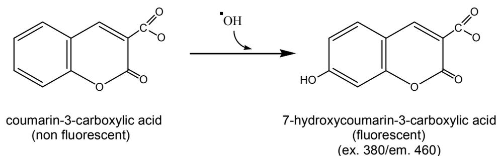
**Figure 5.** Hydroxylation of coumarin-3-carboxylic acid to the fluorescent 7-hydroxycoumarin-3-carboxylic acid (7-OHCCA).
