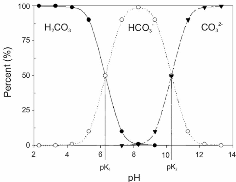
Figure 4. The distribution of carbonate species as a fraction of total dissolved carbonate in relation to solution pH.
