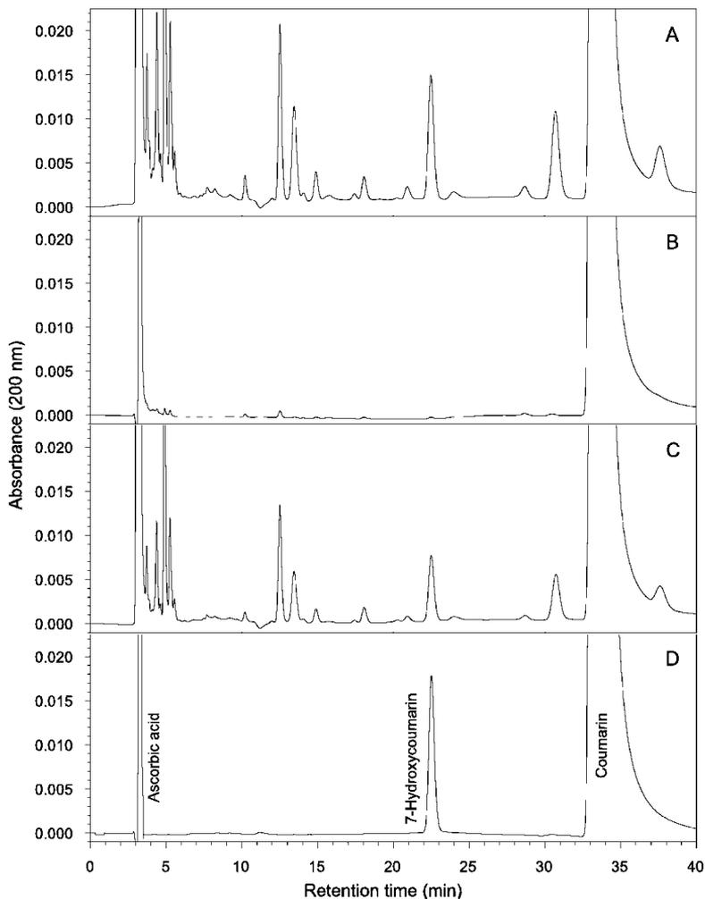
Figure 2. HPLC analysis of ascorbic acid induced hydroxylation of coumarin ( $100\ \mu\text{M}$ ) in the presence of copper or iron. 2 mM ascorbic acid was added to Milli-Q water buffered with 100 mg/l bicarbonate containing (A) 0.1 mg/l copper (B) 0.2 mg/l ferric iron. (C) Both 0.1 mg/l copper and 0.2 mg/l ferric iron present. (D) Ascorbic acid standard (2 mM), 7-hydroxycoumarin standard ( $7\ \mu\text{M}$ ) and coumarin standard ( $100\ \mu\text{M}$ ) in Milli-Q water. Reaction time was 3 h.
