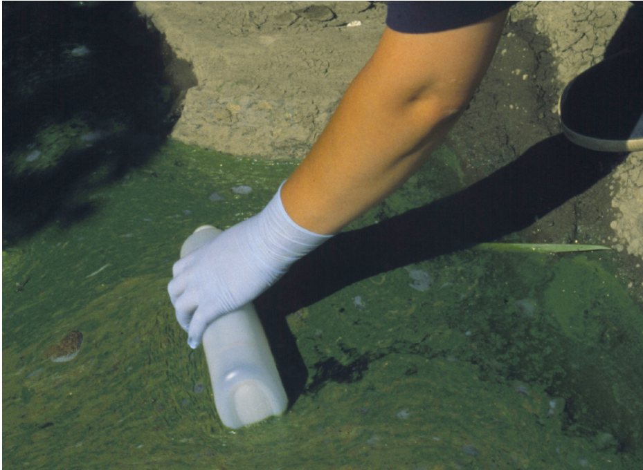
Figure 1.1: Collecting a surface bloom sample of cyanobacteria.
