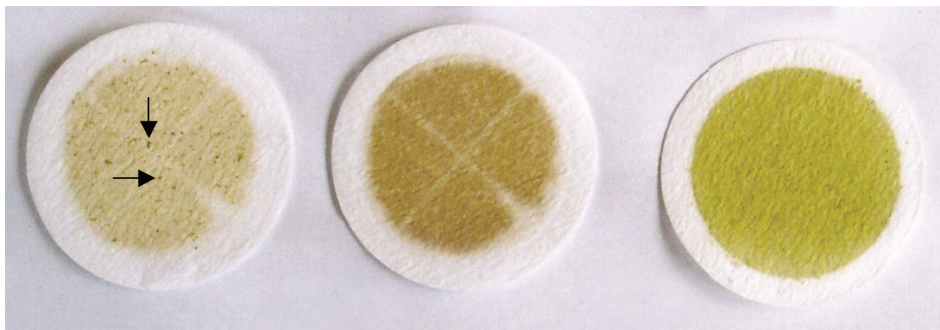
Figure 1.4: Water collected from three lakes with increasing nutrient status (left-right) and filtered onto GF/C filters. The first lake was rich in chrysophytes (left filter), the second in cryptophytes and diatoms (middle filter), and the third in cyanobacteria and green algae (right filter). Single colonies of Microcystis (marked with arrows) can be seen as green spots on the filter to the left.
